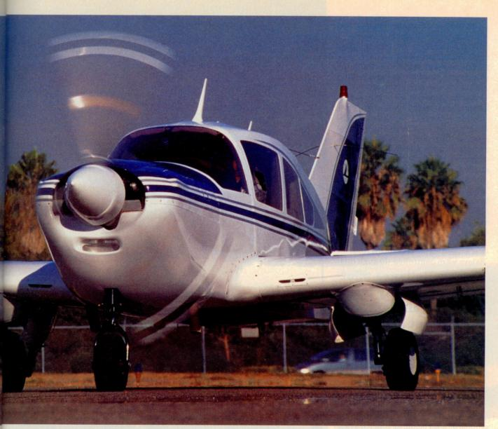
which to choose. Bellanca introduced the Viking in 1967 as the 17-30 with a 300-horsepower Continental IO-520-D. This engine spins at a lofty (and loud) 2,850 rpm for takeoff; maximum continuous power is 285 hp. Two years later,
